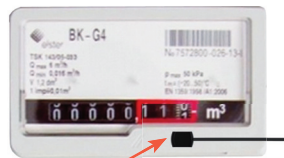
Built-in magnet in the gas meter
